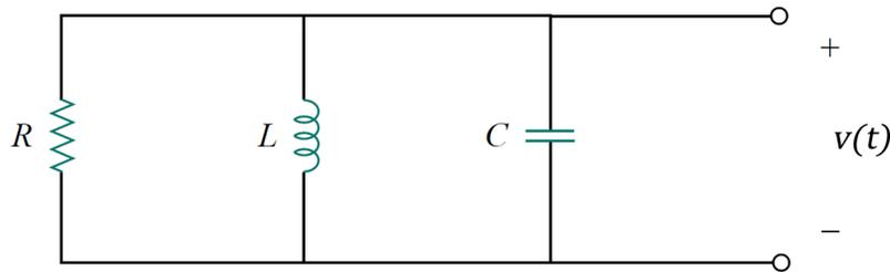
$$V(s) = \frac{s \cdot V_0 - \frac{I_0}{C}}{s^2 + s \frac{1}{RC} + \frac{1}{LC}}$$
