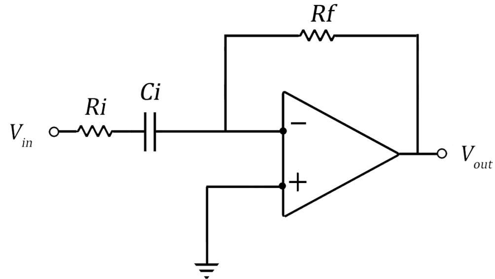
$$R_i = 1K\Omega \text{ , } R_f = 2K\Omega \text{ e } C_f = 10\mu F$$
