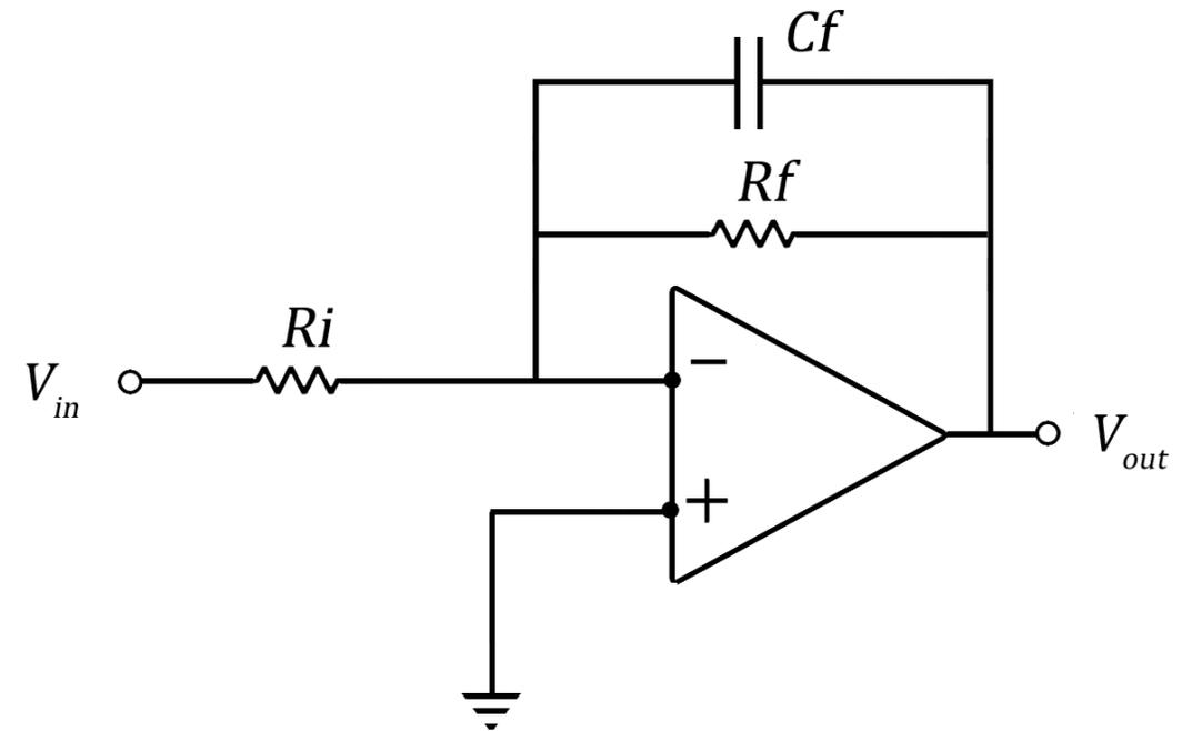
$$R_i = 500\Omega \quad , \quad R_f = 1K\Omega \quad e \quad C_f = 10\mu F$$
